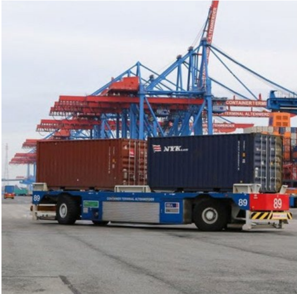
Figure 9: AGV transporting containers from the quayside to the container yard
