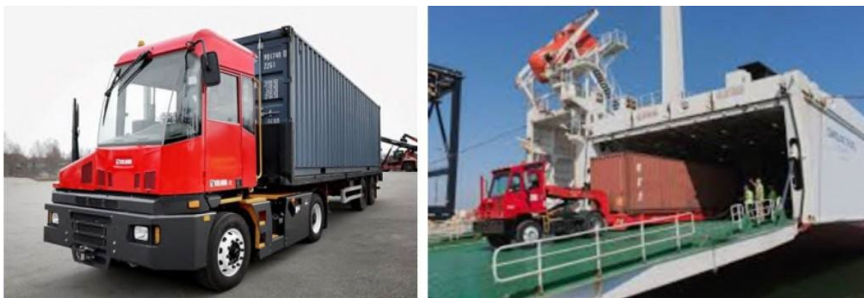
Figure 10: Terminal tractor transporting a container to the container yard (left) and unloading a RoRo vessel (right)
