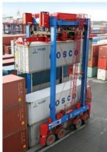
Figure 2: Straddle carrier stacking containers at the container yard
